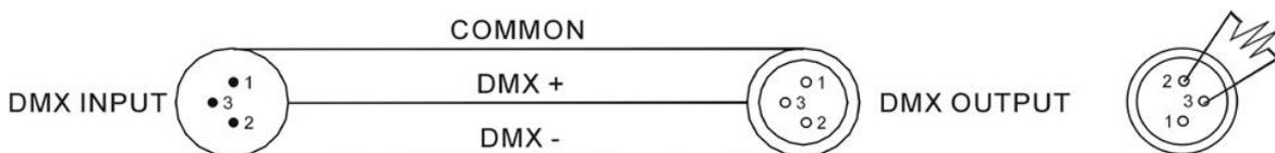
DMX512 is widely used in lamp control, and can control up to 512 channels
