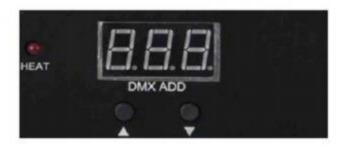
$\Delta$ : Means increasing DMX address code; long press helps increase fast.
