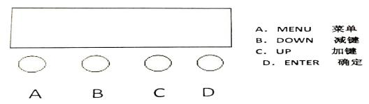
Operating instructions: Press the function key A to cycle out 5 different function effects, the first two digits of the digital tube represent the current function (refer to the function table). The last two digits represent the address code or speed parameter where the function is located. Press B or C key to modify its parameter value. Press D to confirm.
