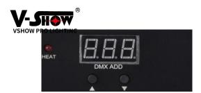
$\triangle$ : Means increasing DMX address code; long press helps increase fast.
