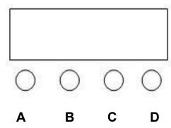
Operating instructions: Press function key A to cycle out eleven different function effects. The first two digits of the Nixie tube represent the current function (refer to the menu). The last two digits represent the address code or speed parameter where the function is located. Press the B or C key to modify its parameter values. Press the D key to confirm
