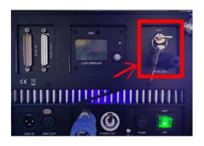
2) When the machine is connected to IDLA line, the system will default to IDLA control mode, and other control modes will not be able to start When using control modes other than IDLA control (such as voice control, self-walking, etc.), the IDLA mode should be adjusted to the closed state in the control panel
